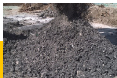
Figure 3 - Dewatered in situ and then remediated using a stabilisation/solidification process
